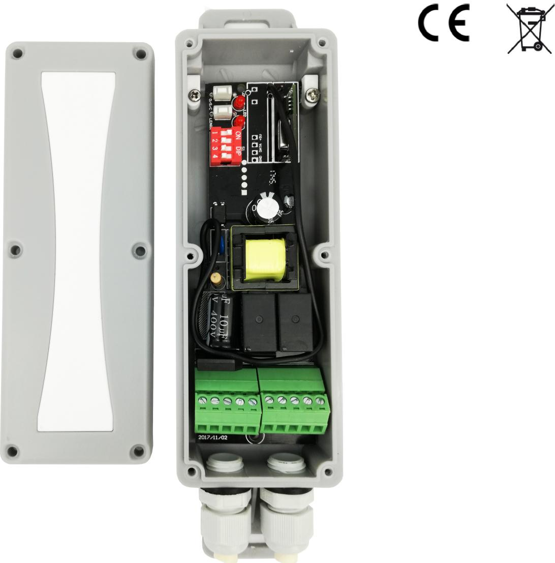
Control board for roller shutters from 100-250V AC, with multibrand and multifrequency receiver RX-Multi integrated (433 MHz frequency). Up/down input switches (configurable as dead man, direct order or sequential switch). Automatic closure and photobeam signal input availables.
